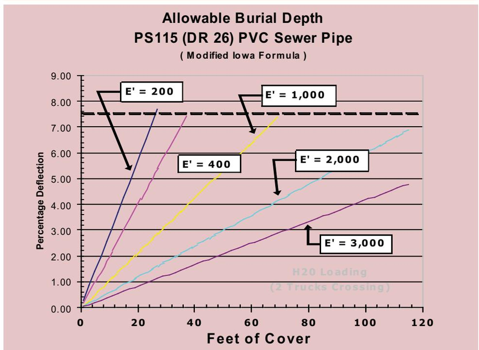
35) pipe can be installed to depths greater than 50 feet. An  $E'$  value of 1,000 psi is easily achieved by placing a graded aggregate material, typically #57 crushed stone or equivalent, around the pipe and to the pipe's springline or above. If higher  $E'$  values are needed, these can generally be achieved by the additional application of slight to moderate compaction.
