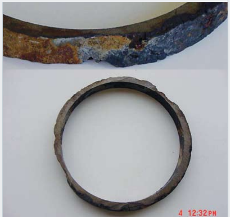
Figure 5, Low Resistivity Clay Soils are Corrosive to Unprotected Iron Pipe (Both photos reprinted from Proceedings of 2007 AWWA Annual Conference , by permission. Copyright © 2007, American Water Works Association.)
