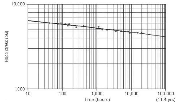
*Note that the line is a result of individual data points (the dots on the figure) – not from loss of strength of a pipe over time.*
