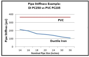
As shown, PVC pipe has higher pipe stiffness throughout the size range and PVC's advantage grows as pipe size increases.
