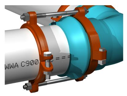
**External Joint Restraint** - These devices clamp to the wall of the pipe and tie back to a mating collar on the fitting or pipe bell.
