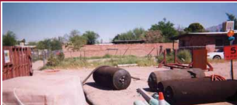
Plugs required for the low-pressure-air test are on-site and available for the acceptance test for system integrity.
