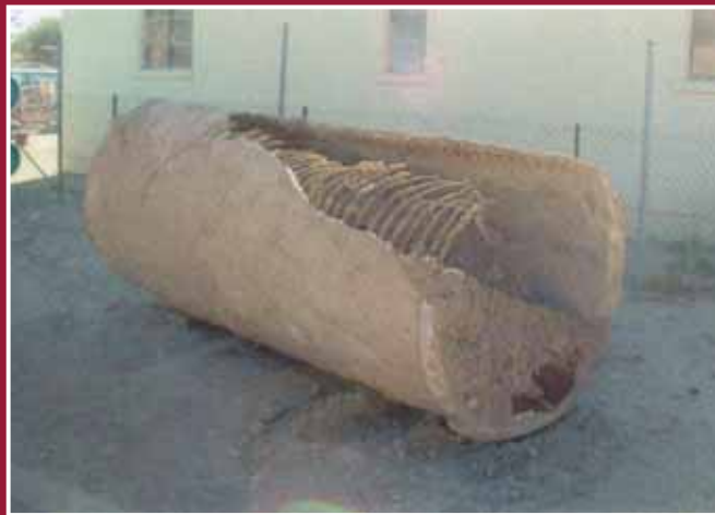
The reason for the sink holes was traced to corrosion at the crown of the concrete sewer interceptor.
