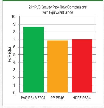
HDPE and PP pipes are subject to strain creep. Strain creep is a property of some materials whereby, when subjected to a load, the pipe will continue to slowly flex under the load over time. For buried HDPE and PP gravity pipes, strain creep means that the pipes will continue to deflect over time. The standards for HDPE and PP gravity pipes make allowances for strain creep over the expected lifetime of the pipes.
