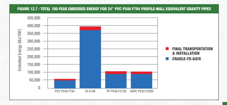
Figure 12.7 compares 24-inch PVC profile-wall, DI, PP and HDPE pipes equivalent to PVC PS46 F794 profile-wall pipe. The total 100-year embodied energy of PVC sewer pipe is 85 percent less than equivalent DI sewer pipe; 44 percent less than PP and 43 percent less than HDPE sewer pipes. It should be noted that the equivalent HDPE sewer pipe has a pipe stiffness that is 26 percent less than the pipe stiffness of PVC pipe.
