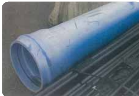
Figure 1: Surface discoloration of PVC pressure pipe stored outdoors, unprotected for 15 years. The discolored pipe passed all test requirements for new pipe.
