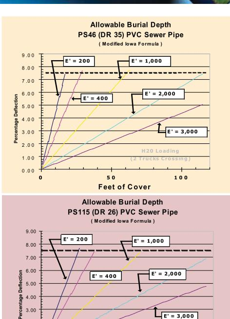
35) pipe can be installed to depths greater than 50 feet. An E' value of 1,000 psi is easily achieved by placing a graded aggregate material, typically #57 crushed stone or equivalent, around the pipe and to the pipe's springline or above. If higher E' values are needed, these can generally be achieved by the additional application of slight to moderate compaction.
