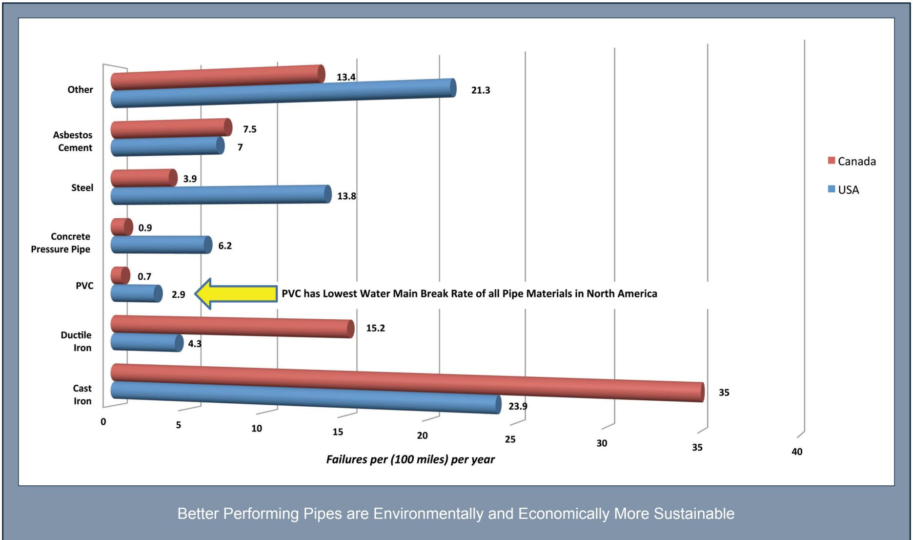
Source: "Water Main Break Rates in the U.S. and Canada: A Comprehensive Study, April 2012" Utah State University, Buried Structures Laboratory
