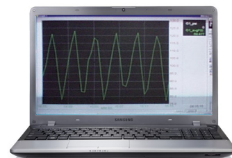
Figure 2: The cyclic pressures applied during testing followed a sawtooth pattern.
