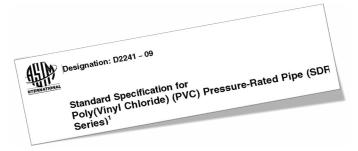
The body of the standard includes IPS (Iron Pipe Size) ODs, while an annex includes Plastic Irrigation Pipe (PIP) and Copper Tube Size (CTS) ODs. Currently there is a project under way at ASTM to add Cast Iron Pipe Size (CIPS) to the annex.
